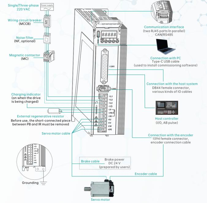
Note: This figure shows the wiring with single/three-phase 220 VAC power supply.
