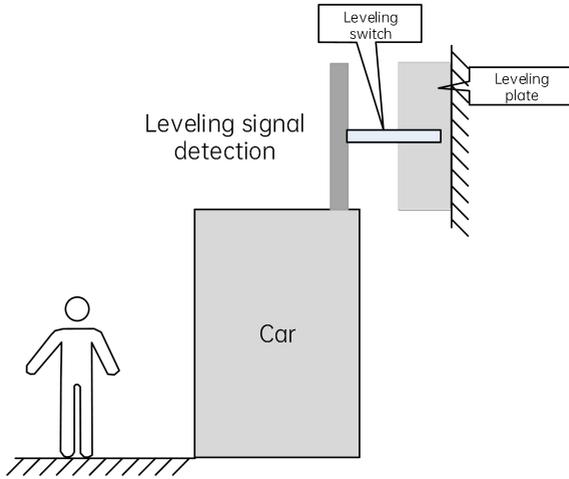
Fig. 3-4 Leveling switch installation position
