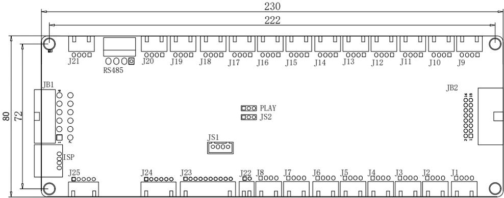
Fig. 10-3 Smile3000-CCB-C terminal layout (unit: mm)
