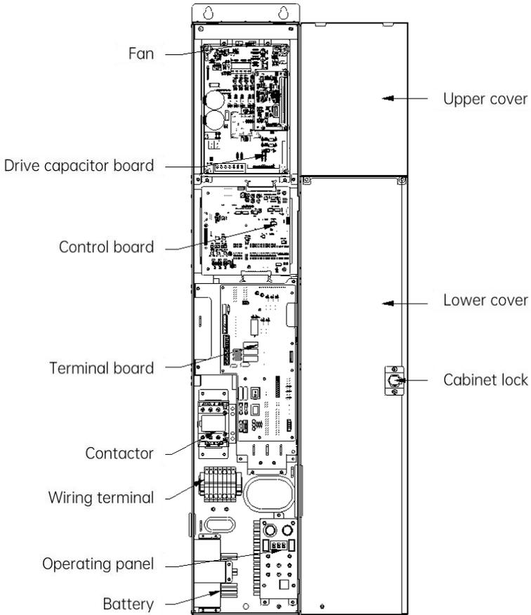
Fig. 2-1 Layout of cabinet top layer
