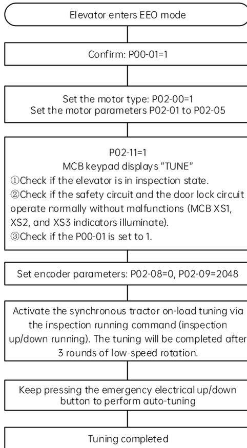
Fig. 6-1 Synchronous motor rotation auto-tuning
