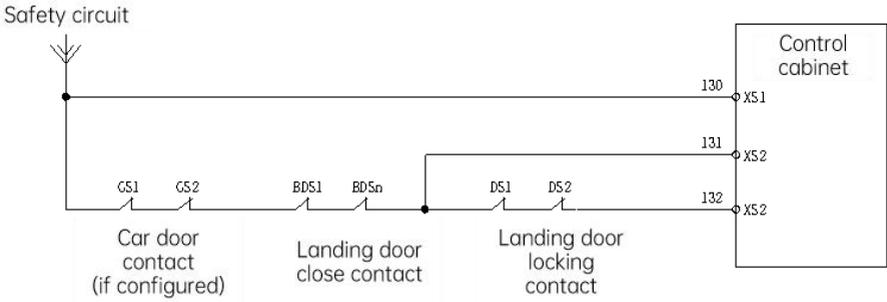
Fig. 11-9 Door lock circuit wiring diagram
