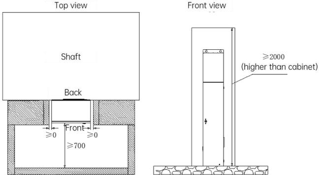
Fig. 3-1 Cabinet installation space (unit: mm)
