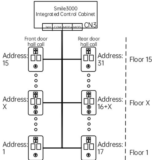
Fig. 11-8 Hall call configuration for 15-floor through-type elevator
