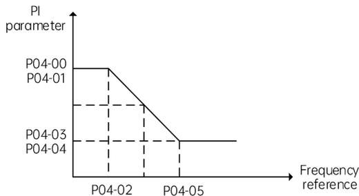
Fig. 7-1 Relation between running frequencies and PI parameters
