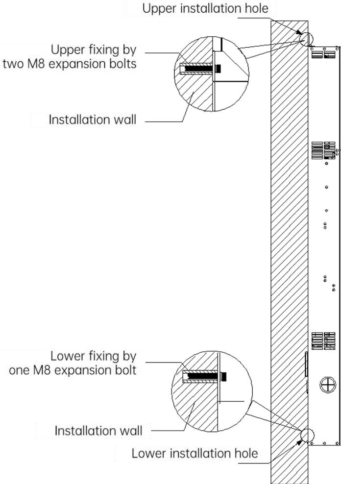
Fig. 3-2 Wall-mounting installation
