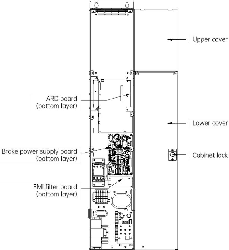
Fig. 2-2 Layout of cabinet bottom layer
