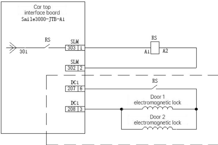
Fig. 11-10 Electromagnetic lock control circuit wiring diagram
