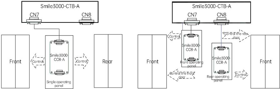
Fig. 11-4 Car call control board wiring diagram
