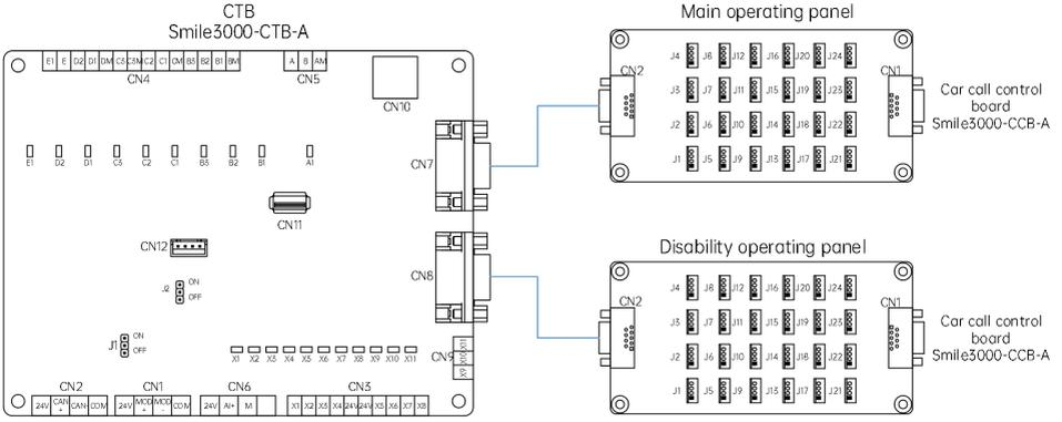
Fig. 11-2 Disability operating panel wiring diagram 1
