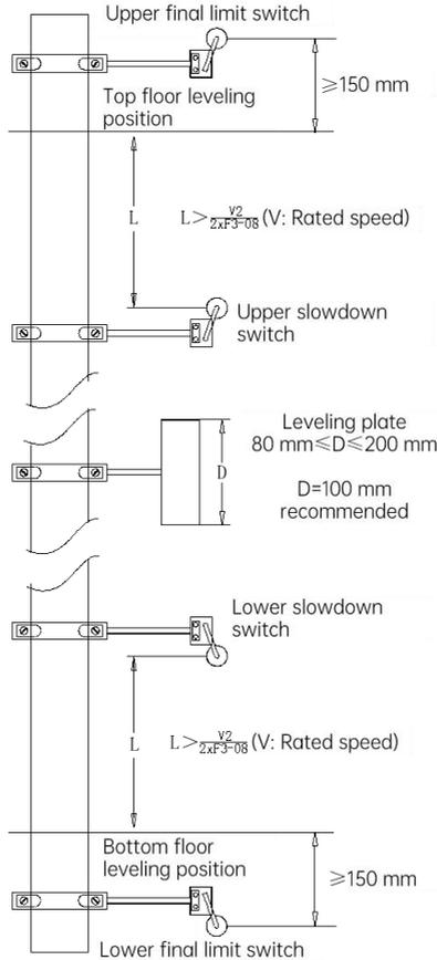
Fig. 3-3 Shaft position switches
