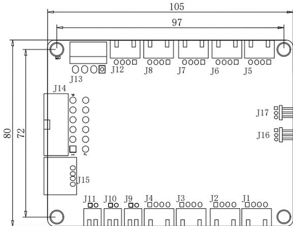
Fig. 10-4 Smile3000-CCB-D dimensions and terminal layout (unit: mm)
