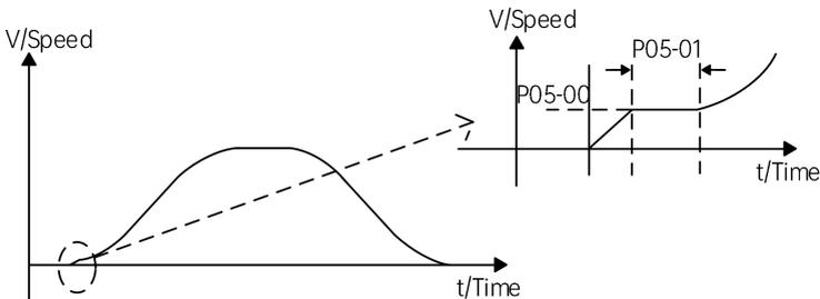
Fig. 6-3 Startup time sequence to minimize static friction influence
