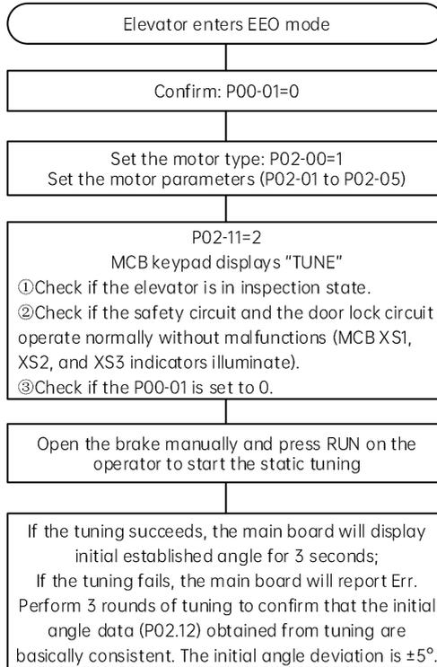
Fig. 6-2 Synchronous motor static auto-tuning
