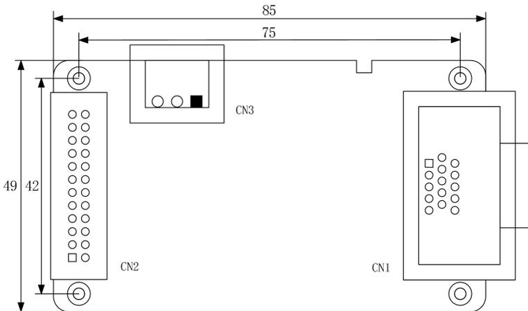
Fig. 4-2 Smile3000-PG-S card appearance and dimensions (unit: mm)
