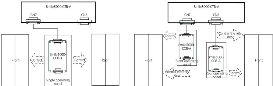
Fig. 11-6 Car call control board wiring diagram of mode 1/2/3
