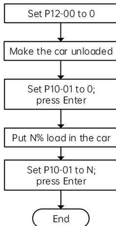
Fig. 11-1 Analog full-load/overload auto-tuning flowchart
