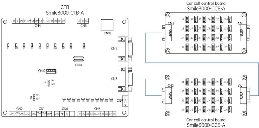
Fig. 11-3 Disability operating panel wiring diagram 2
