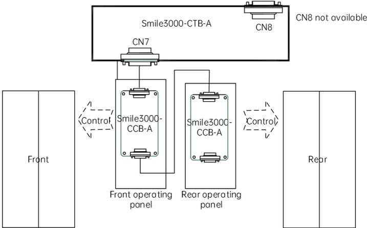
Fig. 11-7 Car call control board wiring diagram of mode 4
